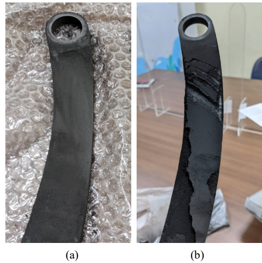
Fig.4. Oxidized connectors made of (a) SG-12 and (b) CG-T.
